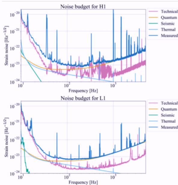
Figure 4: The noise curves of Hanford and Livingston observatories [7]
