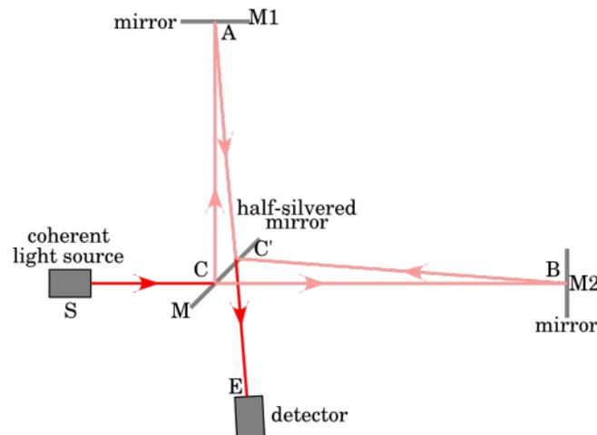
Figure 2: The structure of a Michelson interferometer [3]
